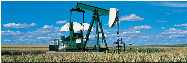
Oil pumpjack in Alberta
